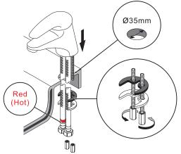
8 Screw the supply hoses on the angle valves.
