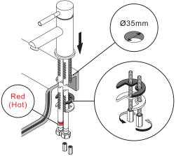
8 Screw the supply hoses on the angle valves.
