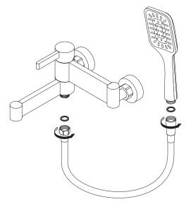
Turn on the faucet and diverter, check for leakage.
