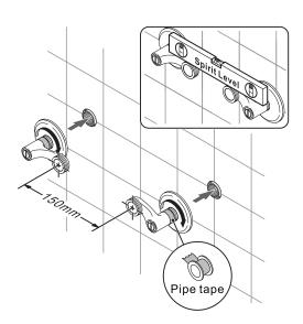
(3) Install the decorative covers on the wall. Put the rubber washers into faucet adapter. Install the faucet on S-connections.
